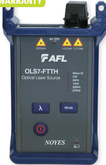
OLS7 Optical Laser Source
